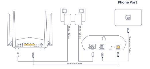
**Tenda V12** Please plug into the yellow port number 4 nbn® Fibre to the Curb installed NCD Please plug into the Gateway port
